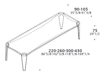
Options: W220 + D90 + H75 W260 + D90 + H75 W300 + D105 + H75 W430 + D105 + H75
